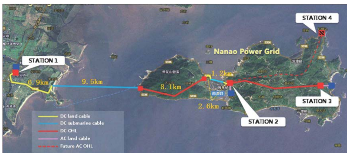
Figure 1 Configuration of Nan'ao VSC project
