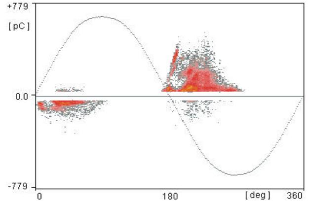
Figure 6: EPR cable - delamination of semicon layer
