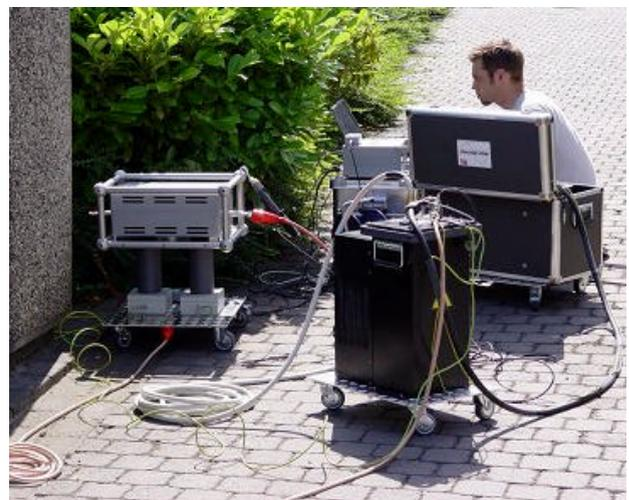
Figure 11: TCC45 - setup with a 60kV<sub>peak</sub> VLF unit
