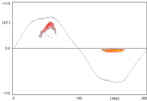
Figure 9: Point-plane discharge starting from a metallic tip
