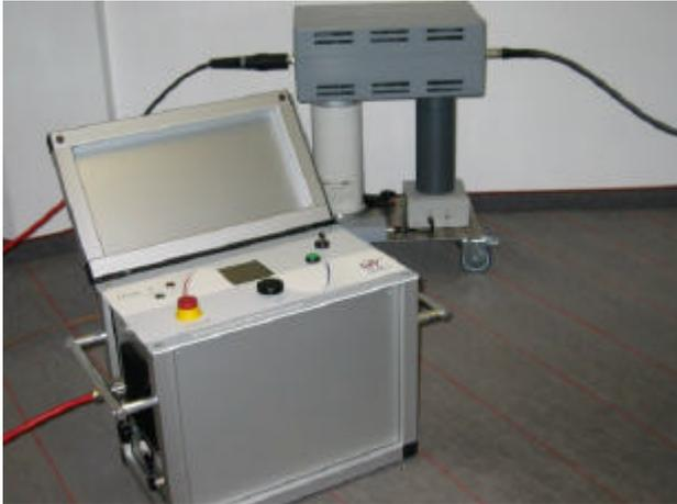
Figure 12: TCC25 together with a 30kV<sub>peak</sub> VLF unit
