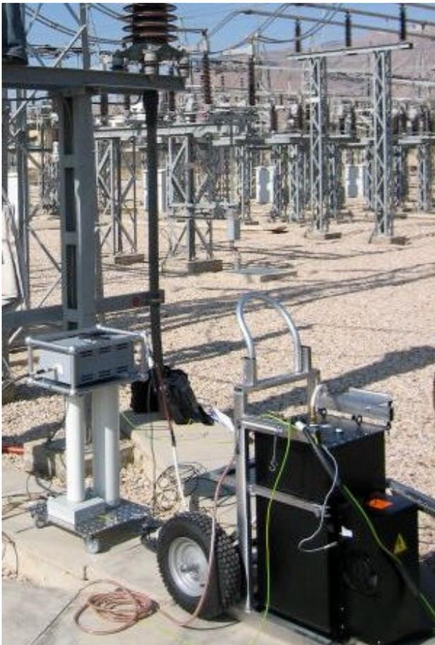
Figure 10: Setup in a substation with a 90kV<sub>peak</sub> VLF unit
