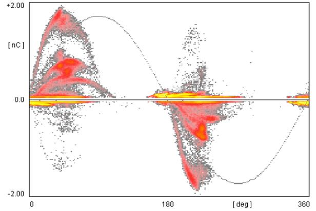
Figure 5: Partial discharge with a cable termination
