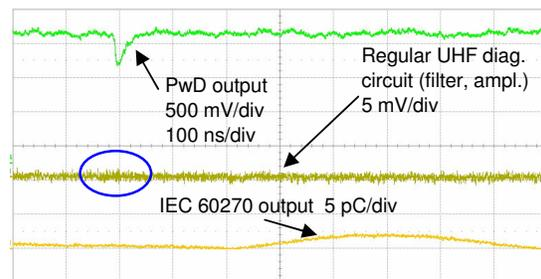
**Figure 10: Sensitive measurement with the PwD, regular UHF and according to IEC 60270 (3 pC)**
