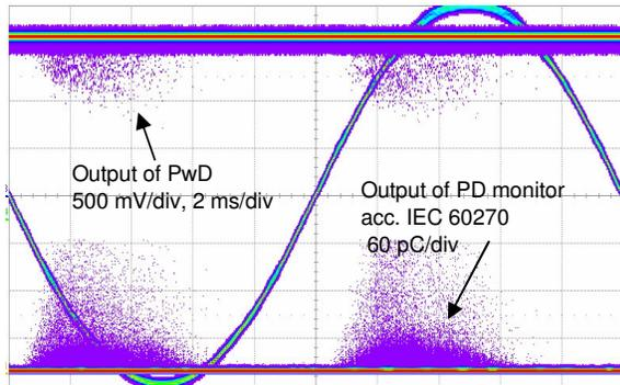
**Figure 11: Phase resolved PD measurement carried out with the PwD comparing to the conventional testing**
