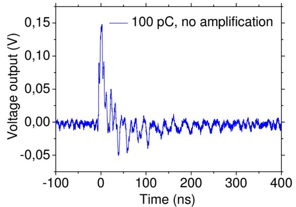
**Figure 13: Output of the voltage sensor at 100 pC**
