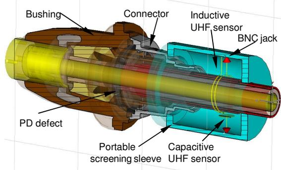
**Figure 1: Object and principle of the UHF diagnostics**
