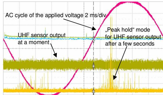
**Figure 9: Phase resolved UHF PD measurement with "peak hold" function**
