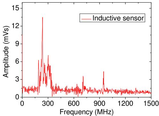
**Figure 5: Frequency spectrum of a PD pulse (15 pC) captured with the inductive sensor in time-domain**
