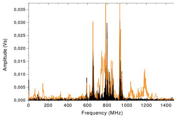
Figure 17: Frequency spectra of the pulse (light curve) vs. background noise (black filled area)
