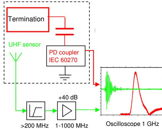
**Figure 6: Structural diagram of the comparative measurement between an UHF and IEC60270 PD detecting methods**
