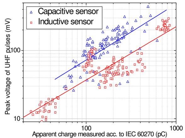
**Figure 7: Sensitivity lines of the UHF sensors (without pre-amplification)**
