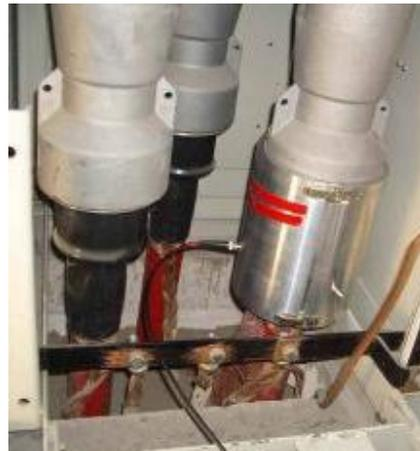
**Figure 15: On-site test set-up: portable screening sleeve with the UHF sensors mounted on each termination in turn**
