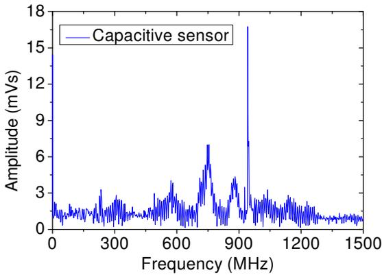
**Figure 4: Frequency spectrum of a PD pulse (15 pC) captured with the capacitive sensor in time-domain**
