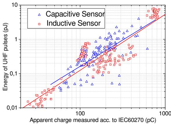
**Figure 8: Correlation between the energy of the UHF pulses and the corresponding apparent charge**
