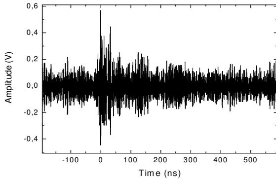
Figure 16: Typical fast pulse emitted by the faulty termination on-site
