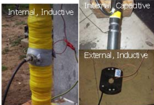
Figure 2: Examples of different sensors to extract the partial discharge pulses from the cable accessories.
