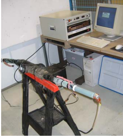
Figure 3: TDS device (ungrounded) developed at IREQ and used for joint characterization
