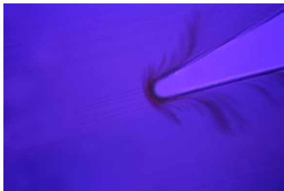
Figure 13: Example of trees growing backwards in copo-XLPE 1. UV micrograph; tree stained with DNPH
