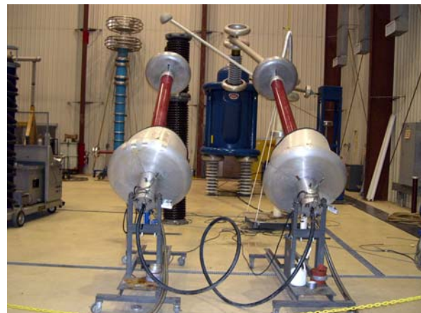
Figure 1 MV cables undergoing ac breakdown testing after long term wet ageing
