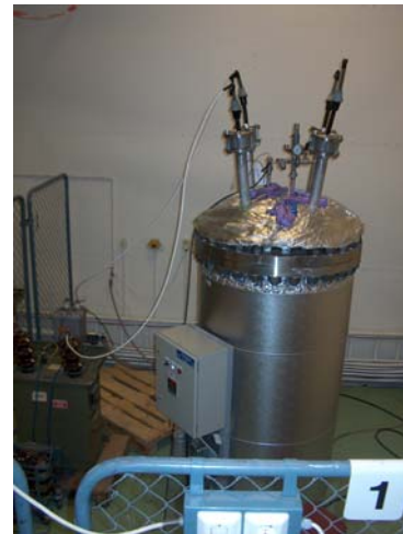
Figure 5: Stainless steel pressure vessel (750 l) for 30 bar long term ageing test.
