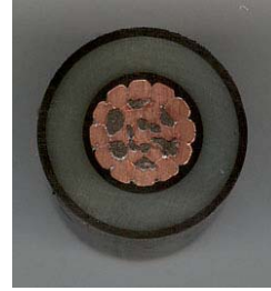
Figure 4: XLPE cable (12 kV cable / 95 mm 2 Cu) used for the water treeing tests – 3.4 mm insulation thickness.
