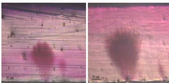
Figure 9 : Water trees grown after submission to electrical stress in 0.1 mol NaCl solution (2 kV RMS, 5 kHz, 24 h) of thermally unaged (left) and thermally aged LDPE samples (95°C, 500 h) (right)
