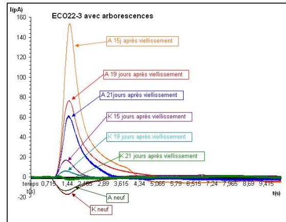
**Figure 14 : Thermal step currents measured on a virgin LDPE sample ("neuf") and on the same sample conditioned at 2 kV RMS, 5 kHz during 48 h in 0.1 mol/l NaCl/water solution. The measurements were made 15, 19 and 21 days after the conditioning.**
