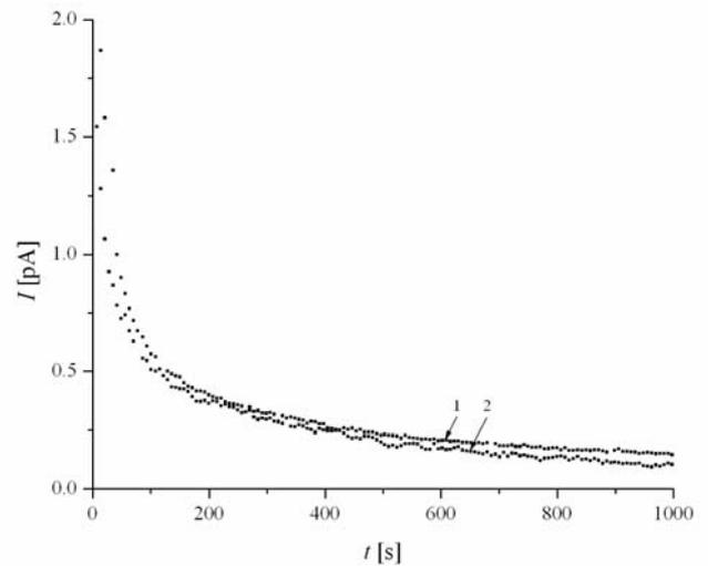
Figure 11 : Absorption currents in a virgin LDPE sample (1) and in a thermally aged sample (105°C, 500 h) (2)
