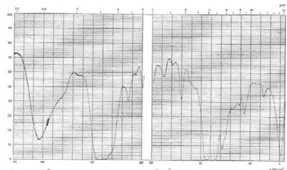
**Figure 6 : Infrared spectrogram of a virgin sample.**
