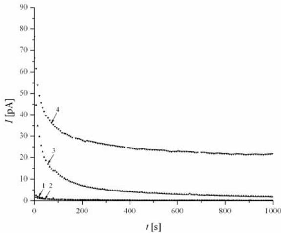
**Figure 12 : Absorption currents in different samples: virgin LDPE sample (1), thermally aged sample LDPE (2), LDPE sample ac-conditioned in 0.1 mol/l NaCl/water solution (3), thermally aged LDPE sample ac-conditioned in 0.1 mol/l NaCl/water solution (4)**
