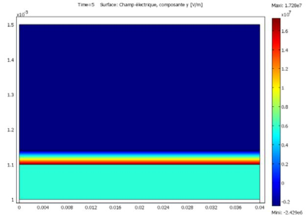
**Figure 17 : Electric field distribution in the case shown in Figure 16**
