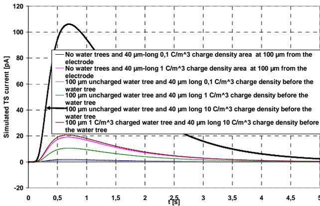
**Figure 15 : Simulated thermal step currents in a water treed sample with different locations of electric charge associated to the water trees**
