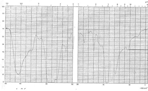
Figure 7 : Infrared spectrogram of a sample aged at 95°C during 500 hours.
