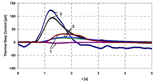
**Figure 13 : Thermal step currents measured on two LDPE samples before conditioning (1), after thermal conditioning in air at 95°C during 500 h (2) and after thermal conditioning in air at 95°C during 500 h followed by ac conditioning at 2 kV RMS, 5 kHz during 24 h in 0.1 mol/l NaCl/water solution (4).**
