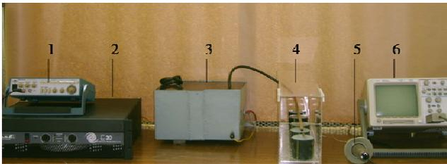
**Figure 4 : Experimental set up for laboratory development of water trees in flat samples: 1- Variable frequency power supply, 2- Amplifier, 3 – 100 V/ 5000 V ac transformer, 4 – 1/1000 high voltage probe, 5 – oscilloscope.**
