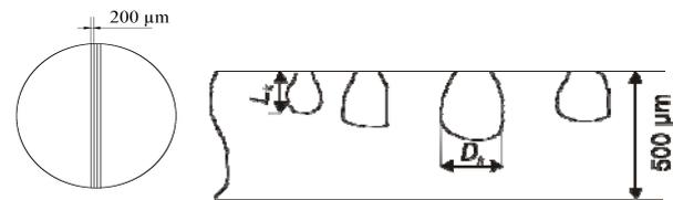
**Figure 5 : Localization and thickness of slices cut for water trees measurement (left) and measurement of the diameter  $D_k$  and of the length  $L_k$  of water trees grown in the samples (right).**
