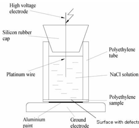
**Figure 3 : Cell used to produce water trees.**
