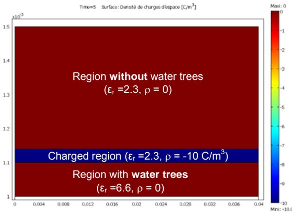
**Figure 16 : Example of a 500  $\mu\text{m}$  LDPE sample containing uncharged water trees and uniformly distributed charge density. If a thermal stimulus identical to that of the measurement bench used in the work is applied in short-circuit conditions to the lower side of the sample, the thermal step current of 105 pA from Figure 15 is obtained**
