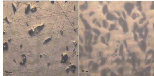
Figure 10 : Defects after pressing in a thermally unaged LDPE sample (left) and in a LDPE sample aged thermally at 105°C during 500 h (right)
