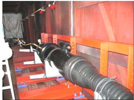
Figure 4: Example of short-circuit test
