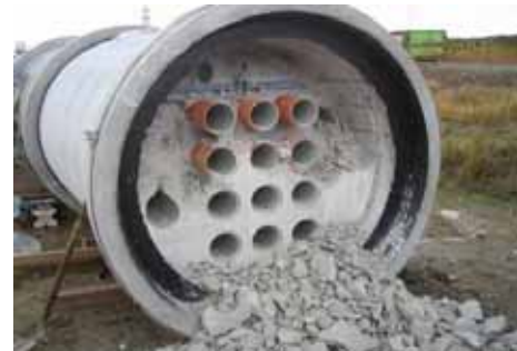
Figure 13: Infill filling state after the full-scale test
