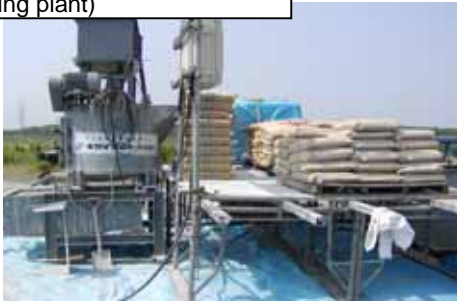
Pressure feed (400 m duct with a diameter of \phi 50 )
