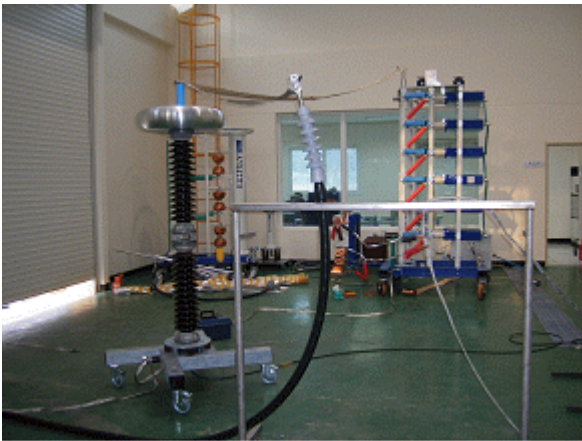
Figure 2: Impulse voltage test setup
