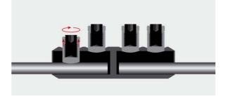
It becomes through the threaded stud tensioned and it stretches axially. On reaching the shear torque it breaks off
