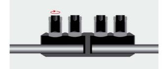
A further screw in of the threaded stud press the shear bolt on the cable
