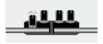
By reaching the contact force, the step less shear bolt blocked.
