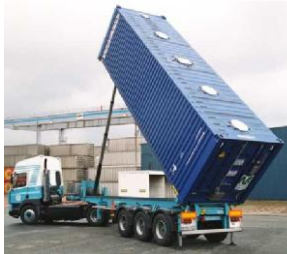
Figure 7. Bulk handling of insulation compound
