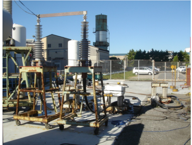
Figure.5 Condition of long-term loading cycle test
