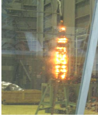
Figure 7: Artificial pollution test
