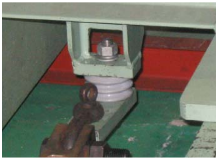
Figure12: Cantilever load test for mounting insulator
