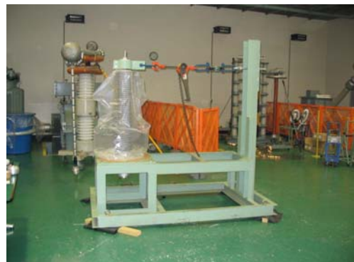
Figure 11: Cantilever load test
