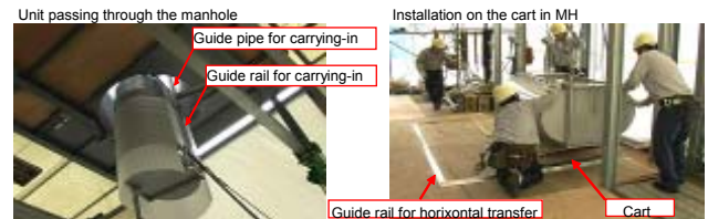
Fig.9. Appearance of carrying test of the epoxy unit into the simulated narrow manhole
