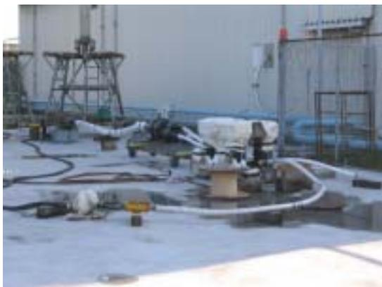
Figure-14. Loading test sample for 77kV 3cDJ
