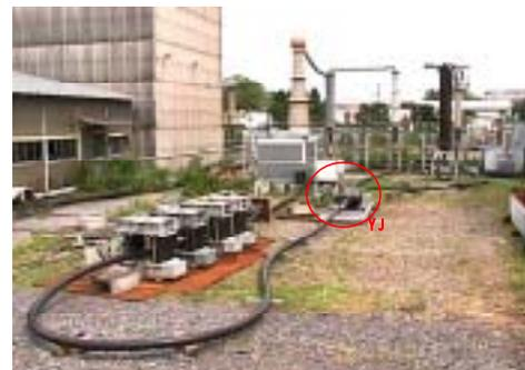
Figure-6. Loading test line for 154kV YJ
