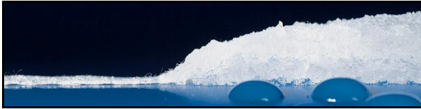
Figure 5: Water blocking tape, dry and wet
