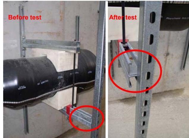
**Figure 7: Movement of the horizontal joint support under the effect of an asymmetric load. (Horizontal joint support and vertical beam not connected)**
