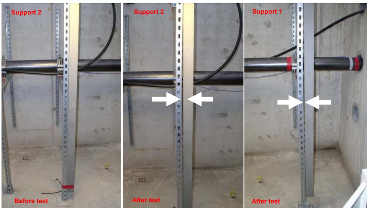
**Figure 8: Bending of vertical beams under the effect of 10 kN asymmetric load (50 – 60 kN).**
