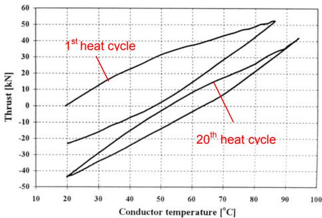
Figure 7: Plot of thrust forces as function of the temperature during heat cycles.
