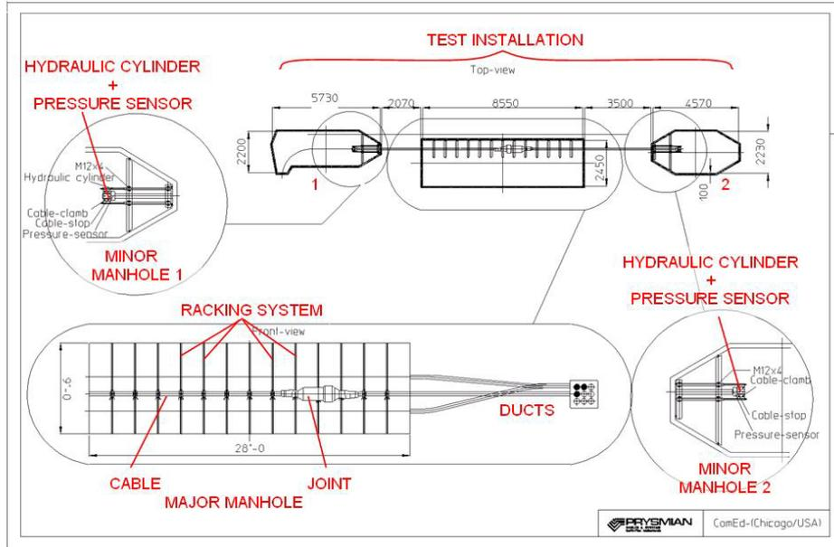
Figure 5: Drawing of the test facility for the characterization of racking systems.
