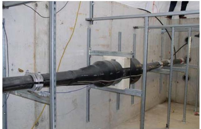
**Figure 4: 345 kV XLPE 1x1600mm<sup>2</sup> Cu (Milliken construction) cable system fixed on the test racking system.**
