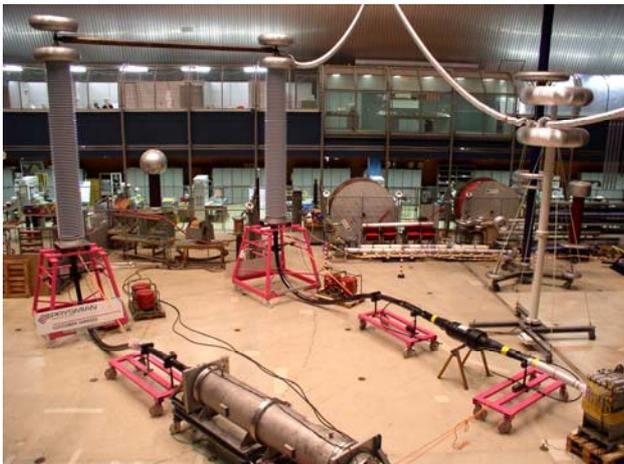
**Figure 3: 345 kV XLPE 1x1600mm<sup>2</sup> Cu (Milliken construction) cable and accessories during type test.**
