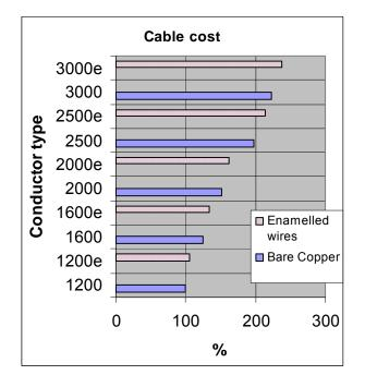
In the above diagram it is shown that conductor from 1600mm<sup>2</sup> to 2500 mm<sup>2</sup> with enamelled wire are less expensive than one cross-section above cables.
