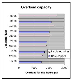
The following hypotheses were taken: Start from maximum load (90°C at conductor). Maximum overload conductor temperature: 100°C. The calculations were carried out according to IEC 60853-2
