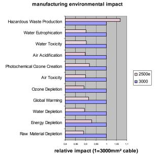
The making of the enamelled cable has globally a lower impact on the environment than the bare copper one. This effect is even more pronounced when taking into account the installation and civil works (smaller cable diameter, longer delivery length). The only drawback at the manufacturing stage regards the hazardous waste production. Although this waste production is very limited. Studies are in progress to reduce it even further.
