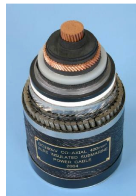
Figure 2: +/- 250kV/180MW HVDC coaxial extruded submarine cable
