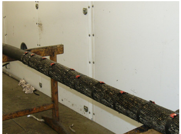
Figure 5. Showing wire to wire welded armouring after restoration
