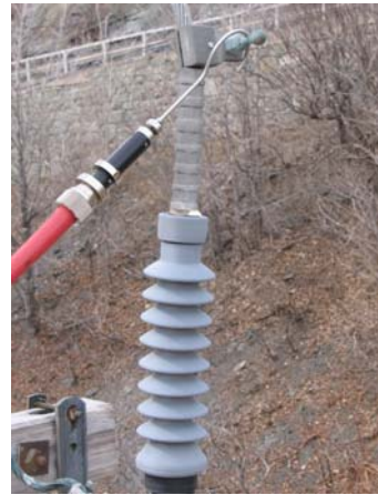
Figure 4: Connector used for the TDS measurement in the field
