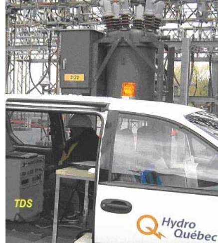
Figure 3: TDS device installed in a small vehicle for field measurements
