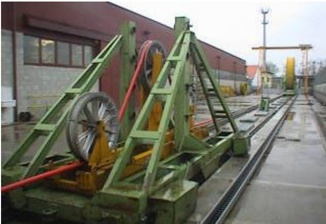
Figure 8. Apparatus for Sidewall Bearing Pressure Testing
