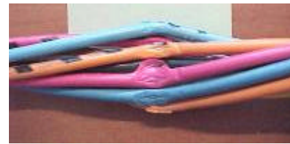
Figure 7. 9/C #12 AWG Insulated Core Removed From Continuous Corrugated Al Armor - 80 Joules Impact
