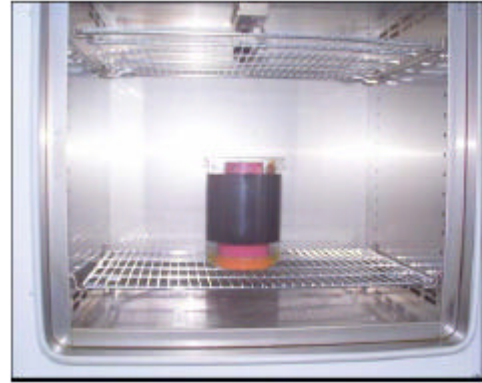
Figure 11. Oil immersion of cable in oven
