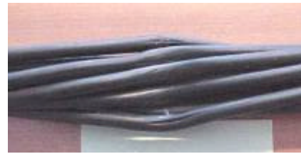
Figure 6. 9/C #12 AWG Insulated Core Removed From Polymeric Armor Design After 80 Joules Impact
