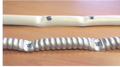
Figure 5. Polymeric Armor and Continuous Corrugated Al Armor – 9/C #12 AWG 600 V Cables - After 80 Joules of Impact and Overall Jacket Removed
