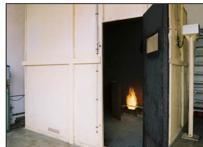
Figure 4: Picture of the smoke opacity 27m 3 chamber
