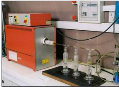
Figure 6: Equipment used for corrosive and acid gas emission test
