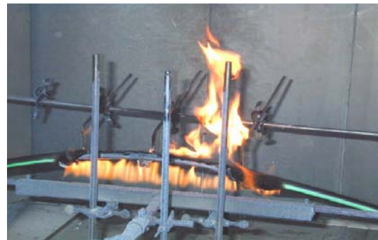
Picture 12: IEC 60331 circuit integrity
