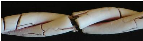
Picture 5: Class 5 insulated conductors / cracks in formation
