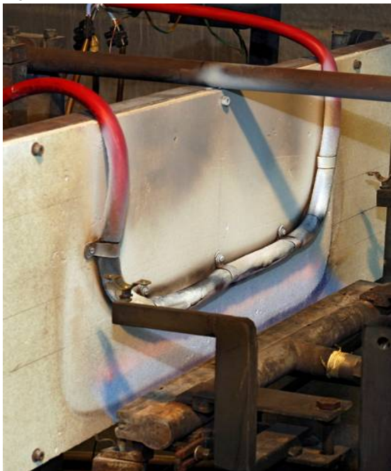
Picture 10: EN 50200 PH 15...120 Circuit integrity with hammer knock
