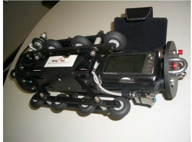
Photo 10: Robotic cable inspection system with digital camera and laser scanning
