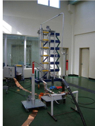
Figure 16: Impulse current test set for arrester
