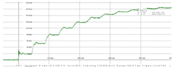
Figure 7: Test result of 350.7m cable line at IVG
