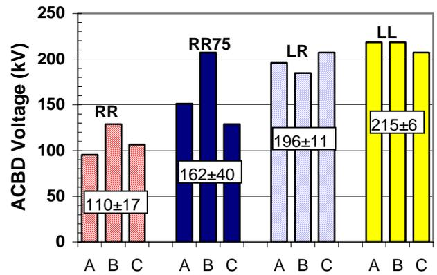
Figure 7 – ACBD voltage of the four cables after thermal cycling with mean value  $\pm$  standard deviation
