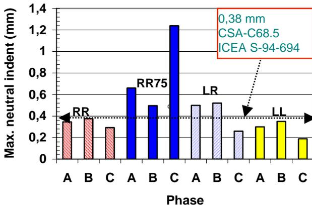
Figure 6 – Maximum neutral indent for the four cables
