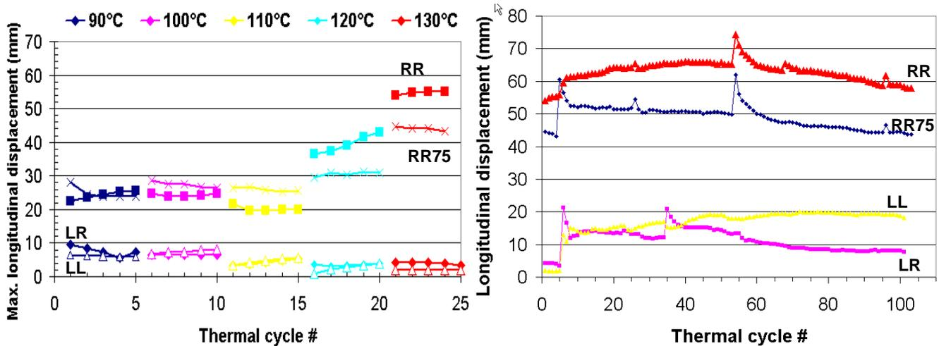
Figure 3 – Longitudinal displacement of the cables at the exit of the conduit in the basement during the first five series of thermal cycles at five temperatures (left) and during all the cycles at 130°C (right).
