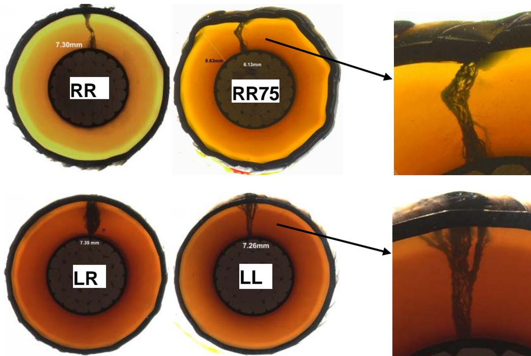
Figure 8 – Slices of each cable showing typical breakdown path after the ACBD test. The insulation thickness is indicated at the breakdown
