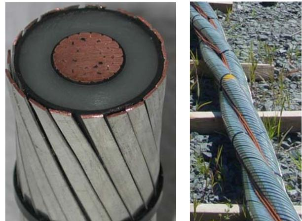
**Figure 1 – Cross-section (left) of the cable with flat strap neutrals, 100% coverage, with a left-hand direction of the lay. Example (right) of the left-hand direction of the triplex assembly for cable LL before installation with the thermocouple wires running in middle.**
