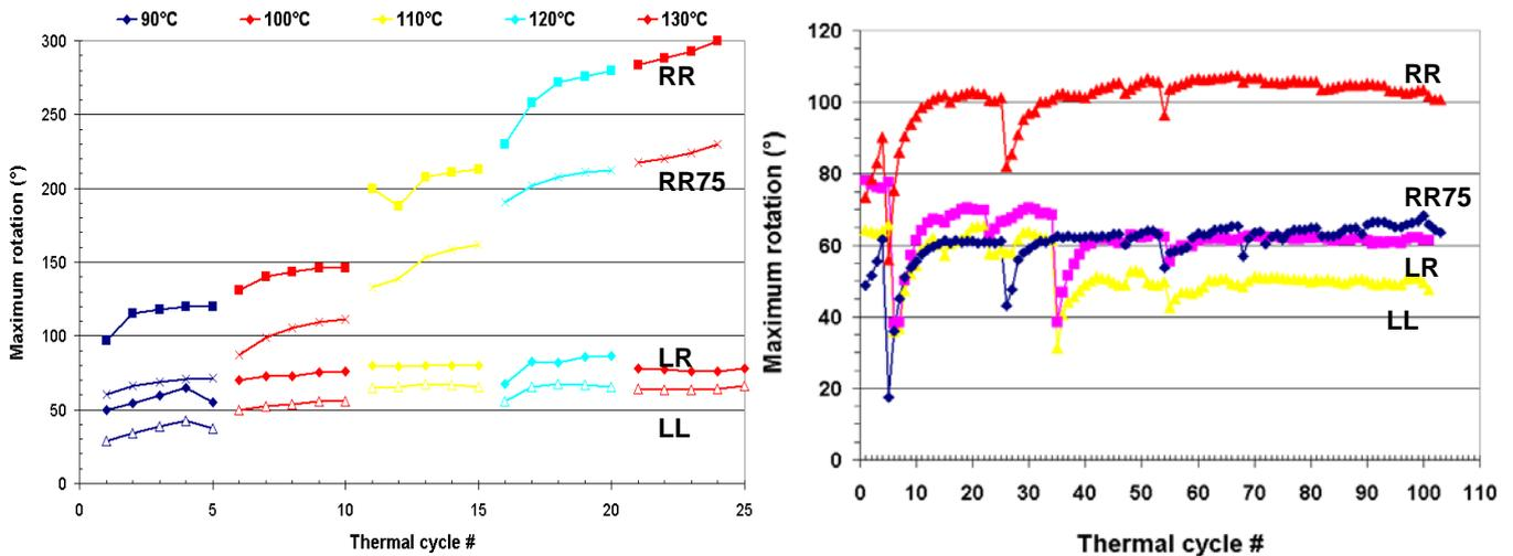
**Figure 4 – Angular displacement of the cables at the exit of the conduit in the basement during the first five series of thermal cycles at five temperatures (left) and during all the cycles at 130°C (right)**
