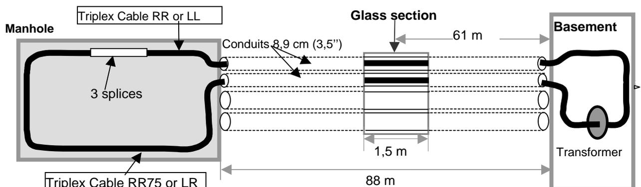
Figure 2 – Diagram of the experimental set-up: underground duct bank extending from a manhole to the laboratory basement
