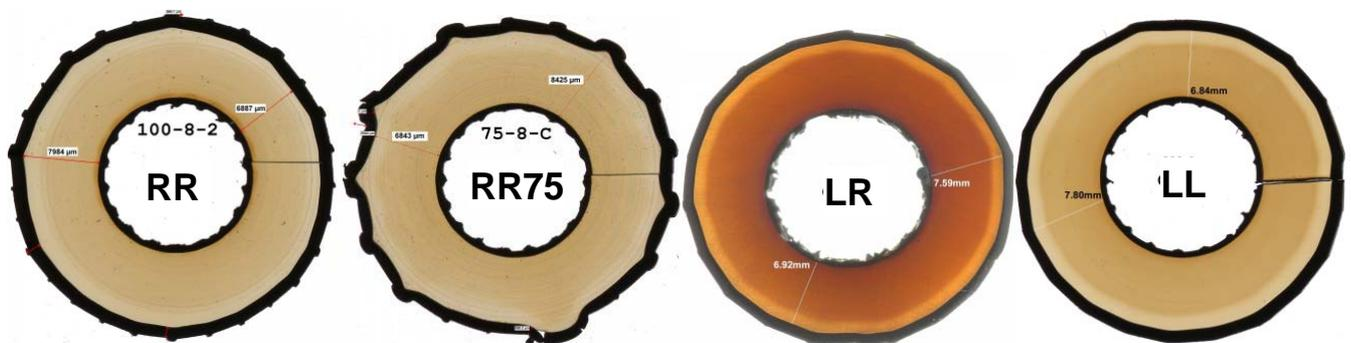
**Figure 5 – Slices of the four cables taken after retrieval in the worst portion, as revealed by the visual inspection**
