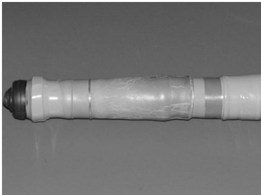
Figure 12: Test sample after tracking resistance test
