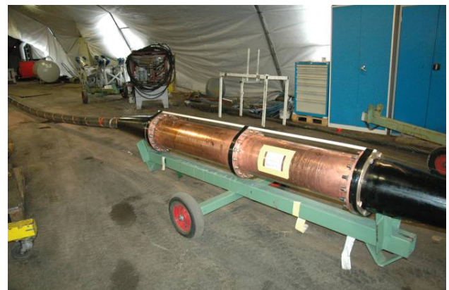
Figure 6. Repair joint ready for mechanical testing.
