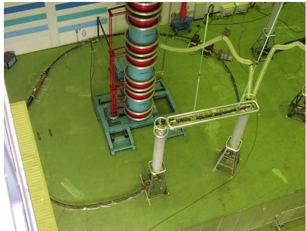
Figure 7. Type test loop in the high voltage laboratory containing submarine cable, repair joint and outdoor terminations.
