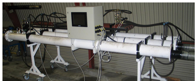
Figure 8. Test rig for fatigue testing of metallic sheaths.
