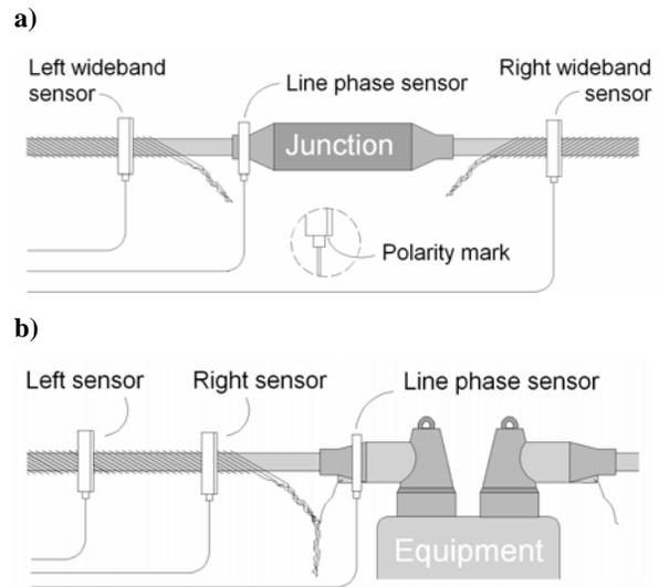
Figure 4: Examples of measuring apparatus on a cable joint (a) and on a unit of equipment (b).
