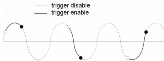
Figure 3: Example of trigger activities controlled by the line phase in order to obtain an unbiased picture of PD phase distribution.
