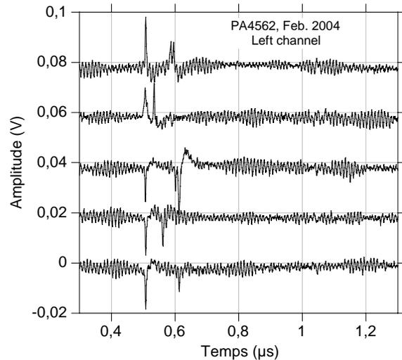
**Figure 6: Examples of closely located discharges taken shortly after that illustrated in Fig. 5. A multiple of a 20-mV step was added to separate the curves. No filter was used.**
