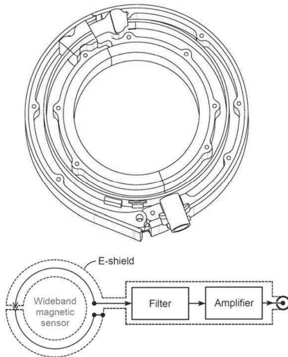
**Figure 1: Wideband magnetic sensor, 3D view (top) and schematic (bottom)**
