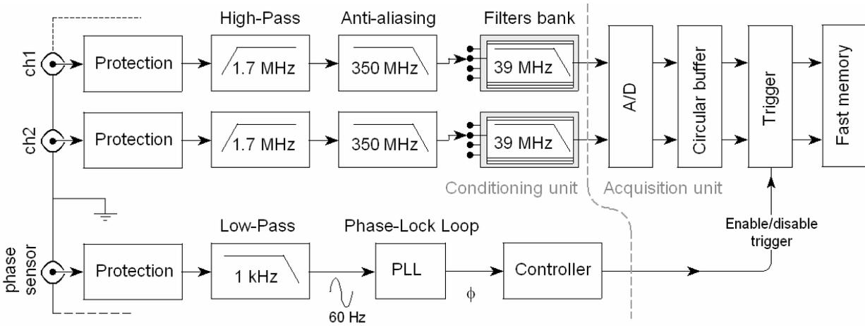
Figure 2: Signal conditioning and acquisition unit.
