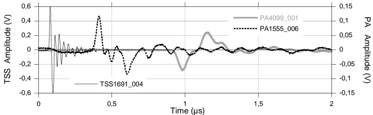
Figure 7: Discharges in a base-mounted transformer (TSS) observed in two manholes, PA1555 and PA4099, located 337 m and 609 m respectively from the transformer.
