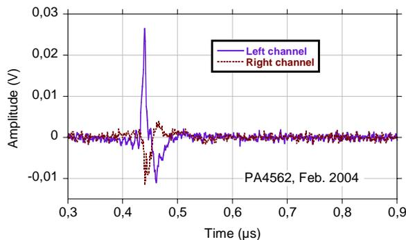
**Figure 5: Discharge in a joint recorded on 19-02-2004 in the PA4562. A digital notch filter is applied.**
