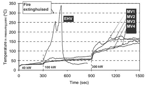
Figure 5 : Temperature measured in the fumes at approximately 8 m from the fire source
