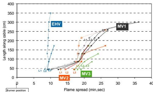
**Figure 9 : Flame spread (min:sec) (X-axis) along the cable length per ladder :**
