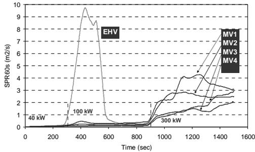
**Figure 6 : Smoke production rate (smoothened over 60 sec) for the tested cables**
