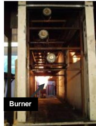
Figure 2 : Experimental set-up of the EHV cable in the horizontal reference scenario (front view)
