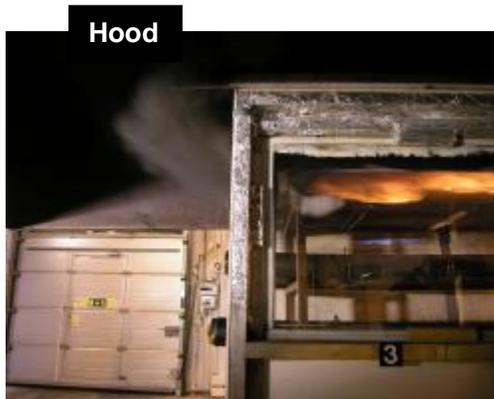
**Figure 7 : Illustration of the smoke production of the HDPE sheathed EHV cable approximately 8 minutes after the start of the test.**
