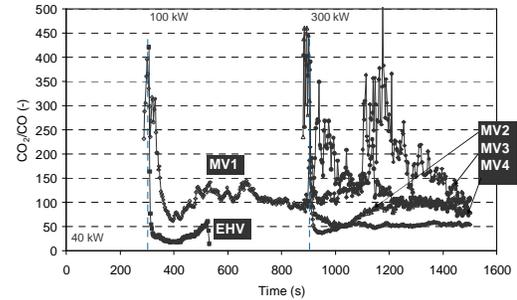
**Figure 8 : CO<sub>2</sub>/CO ratio as a function of time for the energy cable tested. No values are reported from the initial phase of the testing as the CO level (too low) could not be detected accurately.**
