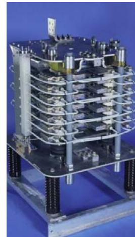
Figure 8: TCR valve (one phase out of three)
