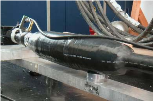
Figure 2: Mounted joint with external screen junction and high frequency current transformers for inductive PD decoupling
