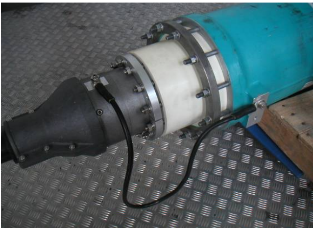
Figure 3: GIS cable termination, detachable
