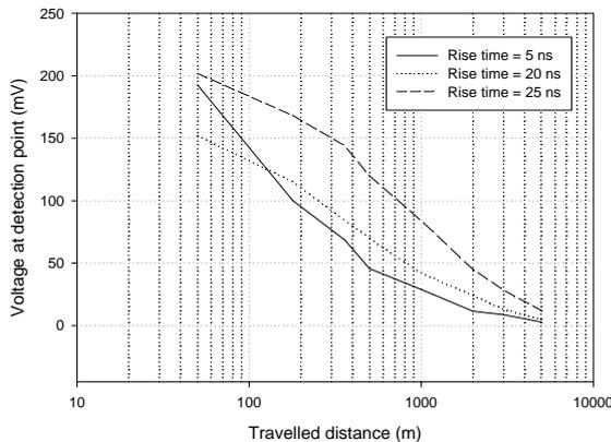
**Figure 10. Simulated PD pulse peak value as a function of travelled distance and for different values of PD pulse rise time. UWB simulation.**
