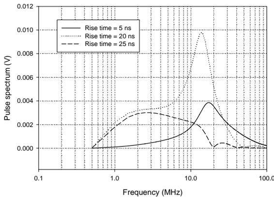
**Figure 9. Measured spectra for calibrator pulses having rise times of 5, 20 and 25 ns.**
