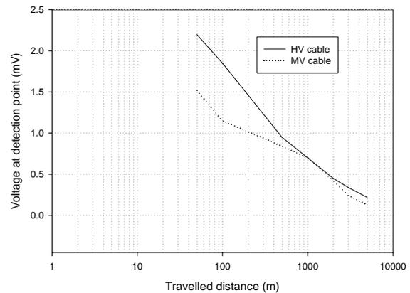
**Figure 8. Comparison between PD pulse UWB detection sensitivity as a function of travelled distance for an XLPE HV cable and a MV cable. Simulation.**
