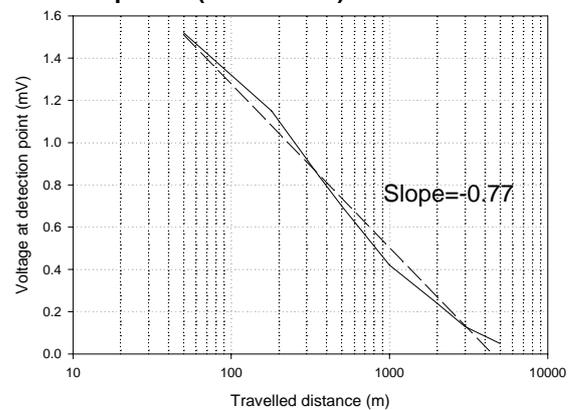
**Figure 4. PD pulse peak value (UWB detector) as a function of travelled distance for a MV cable. The regression line fitting the data is also reported (dashed line). Simulation.**
