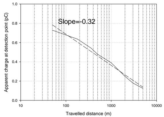
**Figure 3. PD apparent (IEC 60270-compliant detector) charge as a function of travelled distance for a MV cable. The regression line fitting the data is also reported (dashed line). Simulation.**
