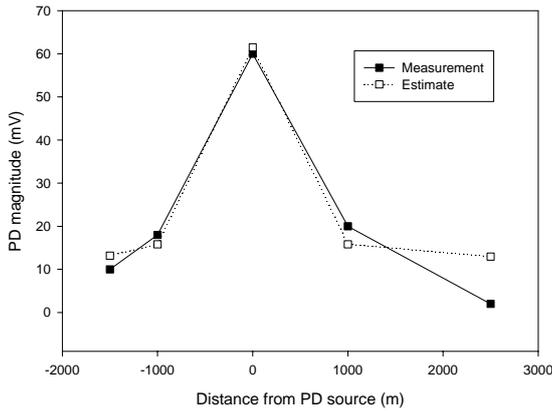
**Figure 6. Comparison between measured and simulated PD height as a function of travelled distance. Measurements come from an after-laying test performed offline on a 220 kV XLPE cable system. PD height at the source has been assumed as the reference value**
