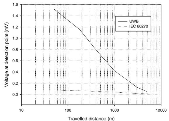
**Figure 5. PD pulse peak value in mV for an UWB and an IEC 60270-compliant detector. Simulation.**
