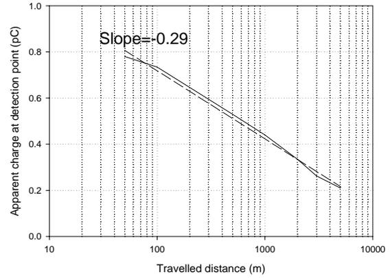
**Figure 7. PD apparent charge (IEC 60270-compliant detector) as a function of travelled distance for a XLPE HV cable. The regression line fitting the data is also reported (dashed line). Simulation.**
