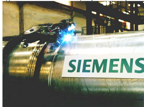
Figure 9: Mechanized Enclosure Welding
