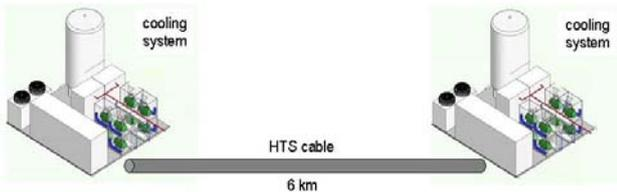
**Figure 10. Cooling systems at both ends of the cable**
