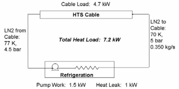
**Figure 11. Schematic for cooling loop for 200 m pilot**
