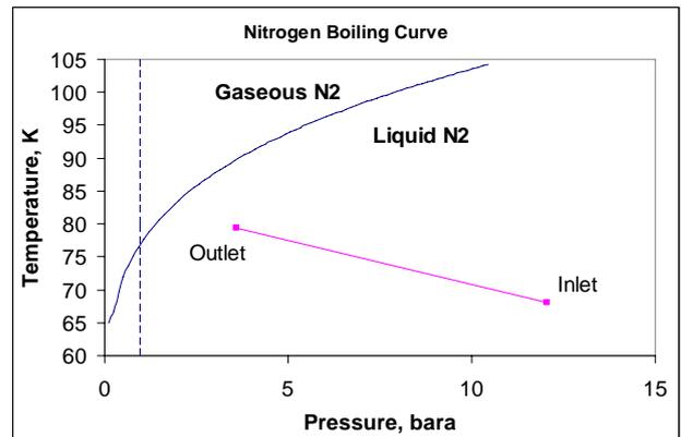
**Figure 12. Inlet vs. outlet fluid conditions for planned cable installation.**
