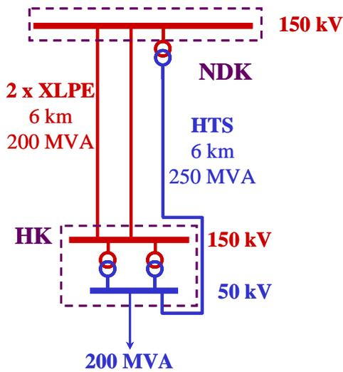
**Figure 5. Network after installation HTS cable**
