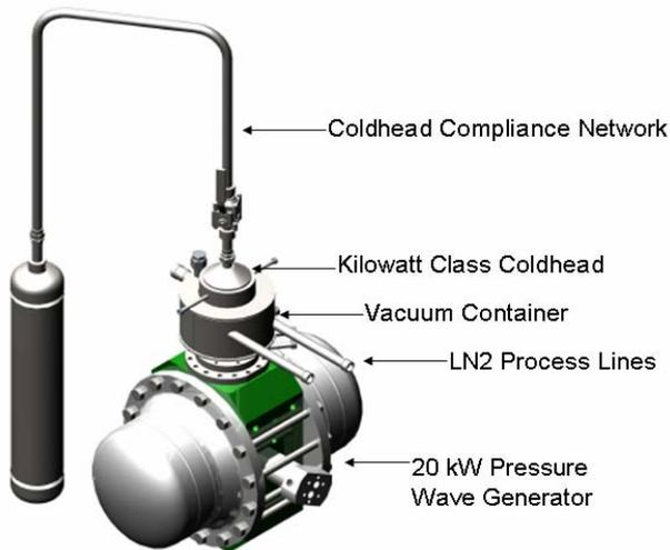
**Figure 13. 1-kW Pulse tube cryocooler design.**
