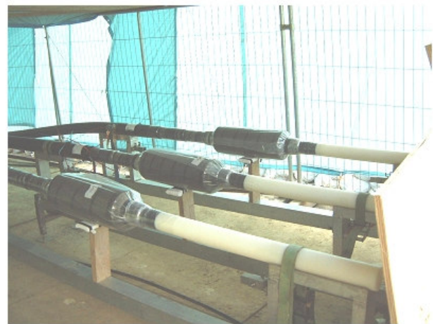
Figure 3: stop joints (blind terminations) used for testing the link in three sub-links
