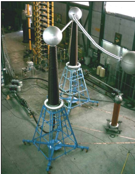
Figure 5: Type test cable loop during withstand test at power frequency
