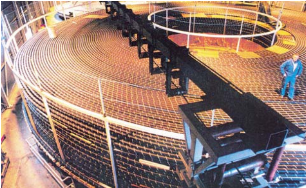
Figure 3: Submarine cable on a turntable (Photo: courtesy of ABB Karlskrona)
