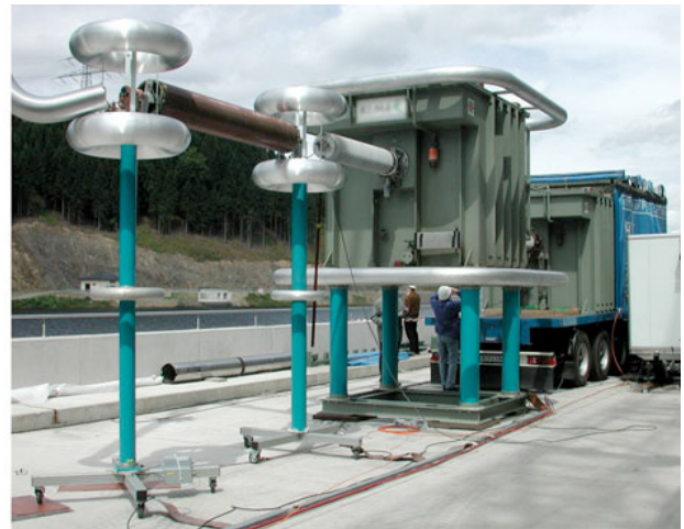
Figure 5: Series connection of two resonant reactors
