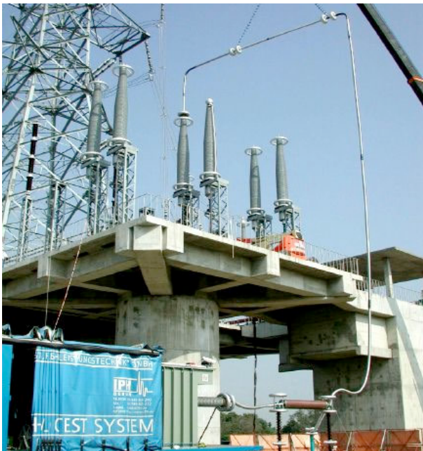
Figure 4: Corona-free test voltage connection
