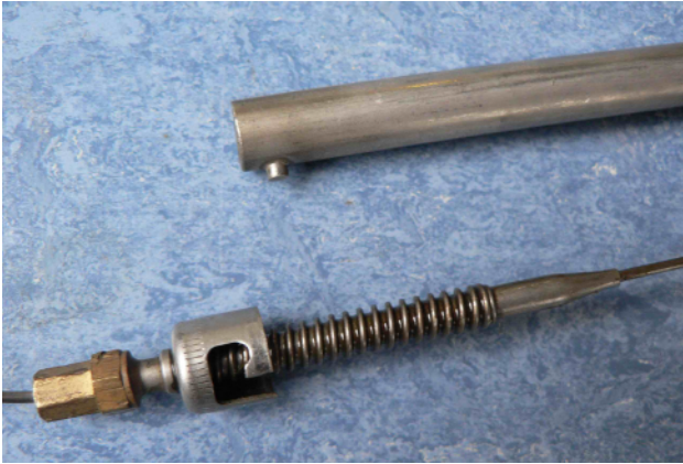
Figure 2 Detail of thermocouple (below) and mounting device (top)
