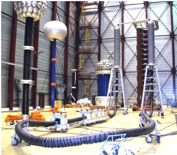
Figure 18 : Lightning impulse tests on a sample taken after load cycling tests
