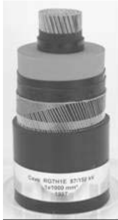
Figure 1: 150 kV EPR insulated cable with tinned copper wires conductor, and copper wires metallic screen wet design
