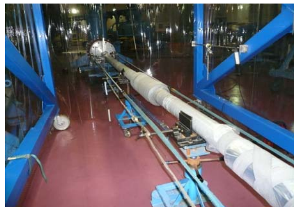
Figure 2. Electrical routine test of a SPJ
