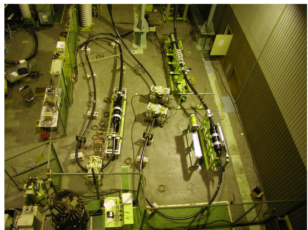
Figure 9: View of Long-term Loading Cycle Test with Thermo-mechanical Test
