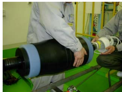
Fig. 17 Assembly of Premoulded Rubber Unit for 400 kV-class CSJ
