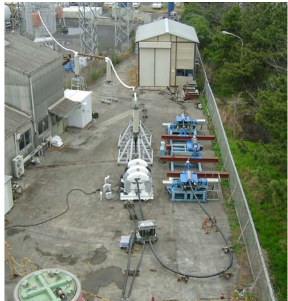
Fig. 19 Test Circuit for Load Cycling and Thermo-mechanical Tests
